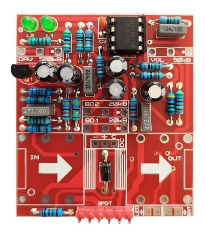
Solder the capacitors, transistors and LED diodes. If you have troubles reading the values, check out our <u>"Reading Part Values"</u> tutorial. Pay attention to the orientation, as well as to the polarity for electrolytic capacitors.
