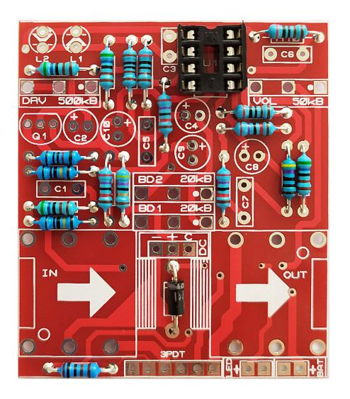
First of all place the IC sockets (without the ICs). Pay attention to the orientation! The small notch in the socket should be oriented as indicated in the PCB.
